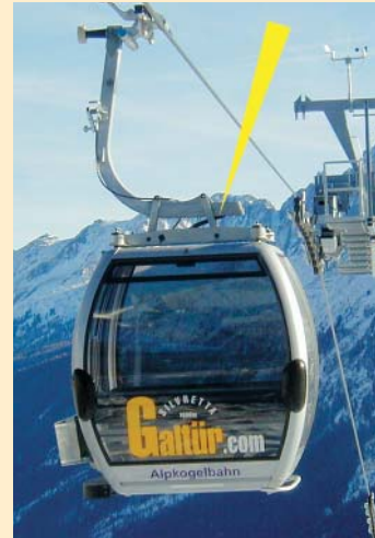
Hydraulic dampers for added convenience when operating cable cars
