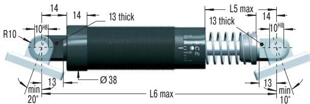
Clevis Mounting Kit C33 = 2 clevis eyes. Delivered assembled to shock absorber. Use positive stop at both ends of travel.
